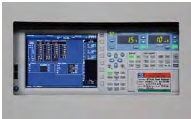
Efficiency determination as per IS 15999 (Part2/Sec1) / IEC 60034-2-1
