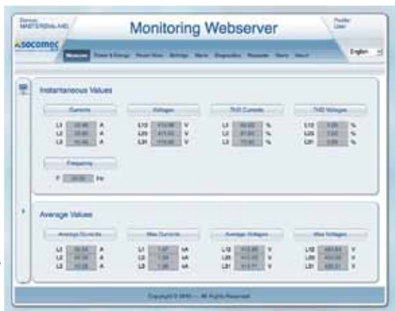
Real-time display of all the electrical values (example screenshot available via the embedded web server function).
