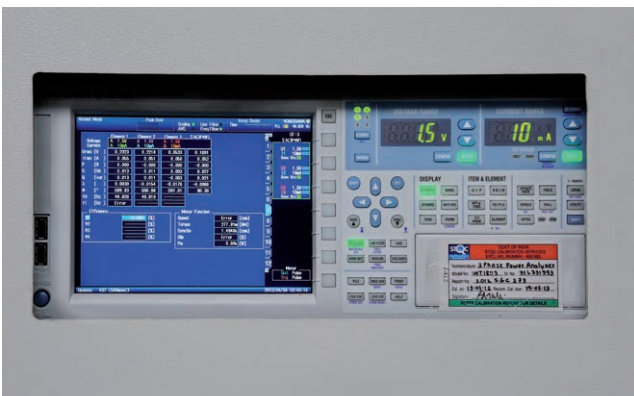
Efficiency determination as per IEC 60034-2-1 IS 15999 (Part 2 / Sec 1)
