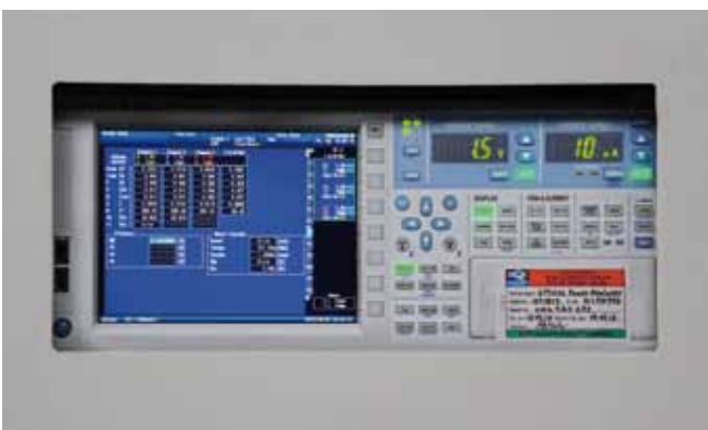
Efficiency determination as per IEC 60034-2-1
