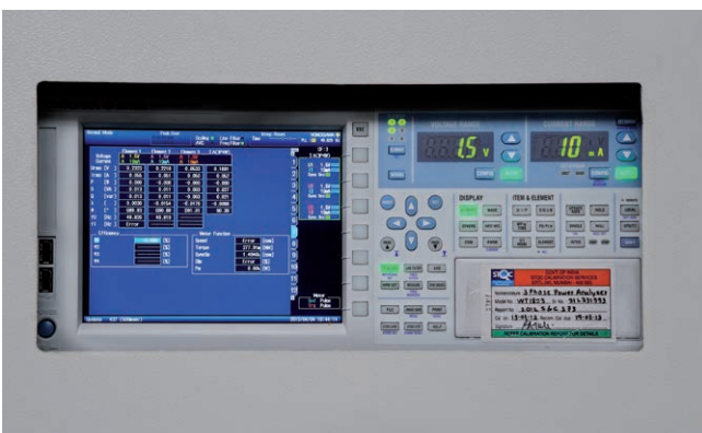
Efficiency determination as per IEC 60034-2-1 IS 15999 (Part 2 / Sec 1)
