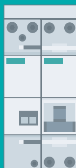
5SM6 AFD unit + 5SY60 MCB = 2 MW
