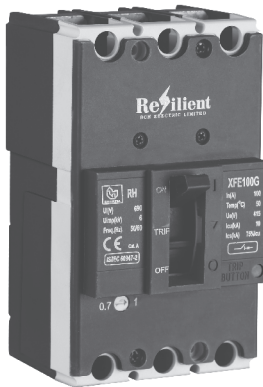
Frame -1 : I_{cu} / I_{cs} = 15/15, 25 / 25, 30/15, 36/30, 50/25 kA
